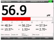
**Digital Display**: shows the instantaneous value of the measured function in form of a large sized numbers with the selected resolution of decimal digits; a coloured bar represents the measured value as a fraction of full scale. Statistical information is given in the lower part of the display.
