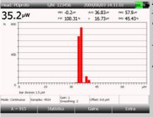
Histogram Display: shows, in form of histogram, the number of times the same value occurs during a measurement session; measured values are shown in the X axis and the number of events in the Y axis. This display is a powerful tool to monitor, e.g., laser sources stability. Instantaneous values are shown in digital form. The vertical scale is automatically adjusted to allow the adding of more data. Statistical information is also given in the upper part of the display.
